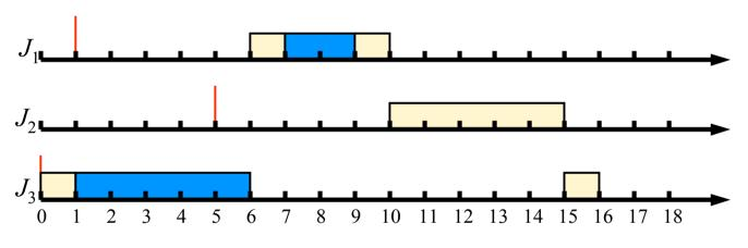
Priority scheduled:  $J_1$  has highest priority. Shading indicates the critical sections, red lines indicate release times for the jobs.
