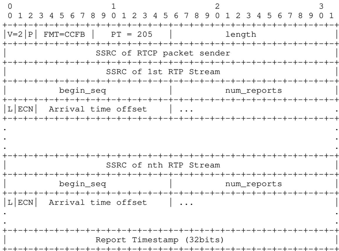
Figure 1: RTCP Congestion Control Feedback Packet Format
