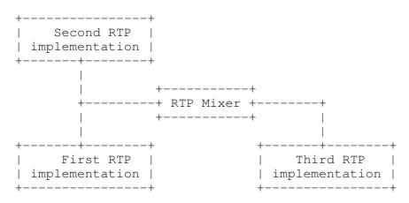
Figure 4: Testing architecture for mixers
