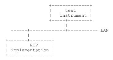
Figure 2: Testing architecture for RTCP
