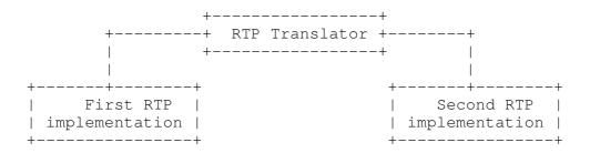
Figure 3: Testing architecture for translators
