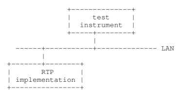
Figure 2: Testing architecture for RTCP
