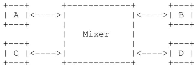
Figure 9: RTP Mixer with Only Unicast Paths
