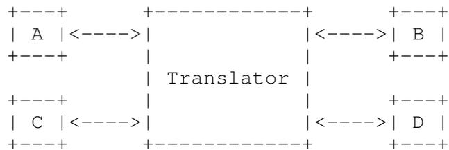
Figure 16: RTP Translator (Relay) with Only Unicast Paths
