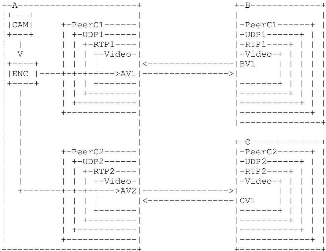
Figure 8: Single Encoder Multi-Unicast Setup
