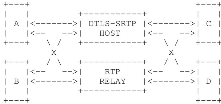
Figure 18: DTLS-SRTP host and RTP Relay Separated
