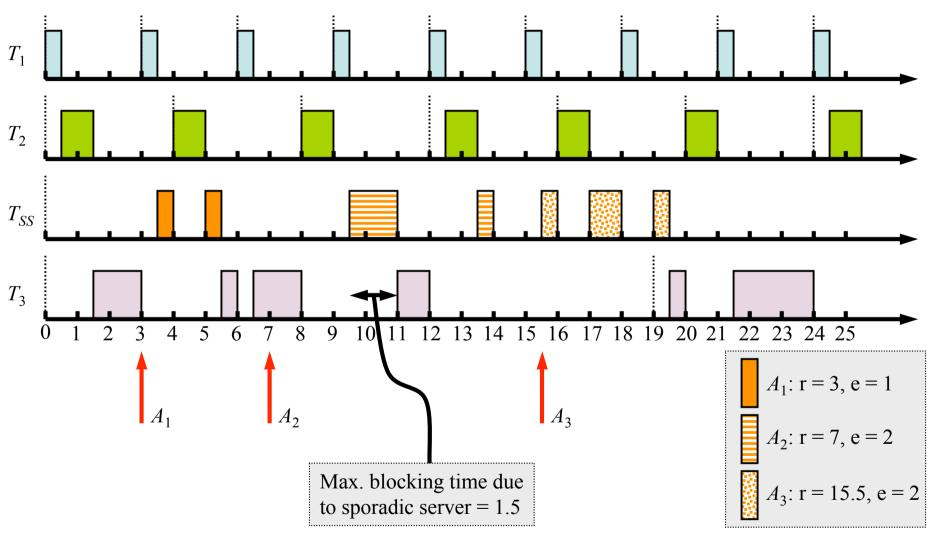
$T_1$ =(3, 0.5),  $T_2$ =(4, 1.0),  $T_3$ =(19, 4.5),  $T_{ss}$ =(5, 1.5) Rate monotonic schedule; simple sporadic server
